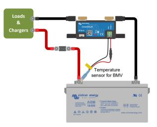
Please note that if the temperature sensor is used, the red power cables that came with the SmartShunt are not needed. The temperature sensor will replace these cables.
