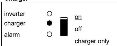
The AC input voltage is switched through and the charger operates in bulk or absorption mode.
