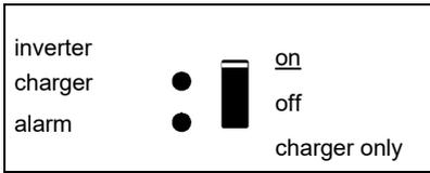
The AC input voltage is switched through and the charger is switched off. The battery charger can not reach battery end voltage (bulk protection mode).
