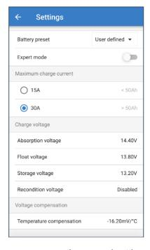
To access the advanced settings menu, open the general settings menu and enable the 'Advanced settings' switch, then select 'Advanced battery settings'.
