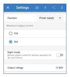
It is also possible to enable low current mode or night mode while in power supply mode and to specify the desired output voltage.
